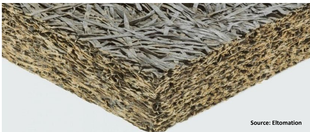
Figure 3.1—Close Up View of Wood Wool Cement Material
