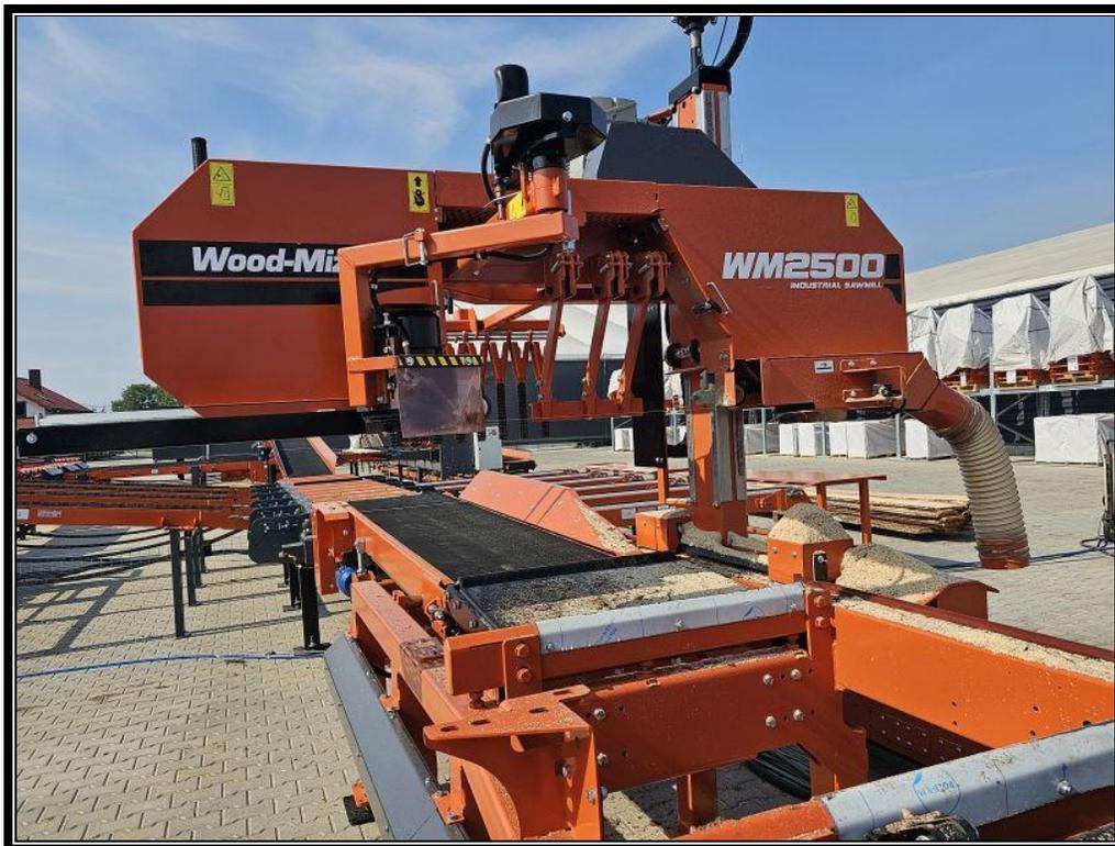
5. *Resaw*—After the primary breakdown squares the log into what is called a *cant* (resembles a roofing beam), the resaw is a secondary piece of equipment that cuts boards and timbers from the cant.
